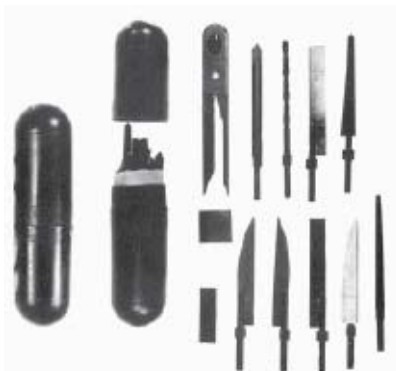
The CIA Escape and Evasion Rectal Suppository was a multipurpose tool kit packed within a smooth waterproof black plastic or aluminum shell; circa 1955 (actual size: 4” long x 1” diameter).
