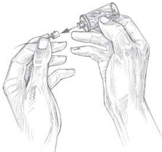
Rigid container showing stopper at top to which thread is attached. Stopper closes top air vent. Exit hole is in center of bottom of container. Phil Franke
