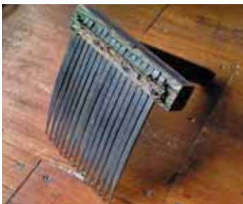
Senbakoki blades on the threshing tool.
