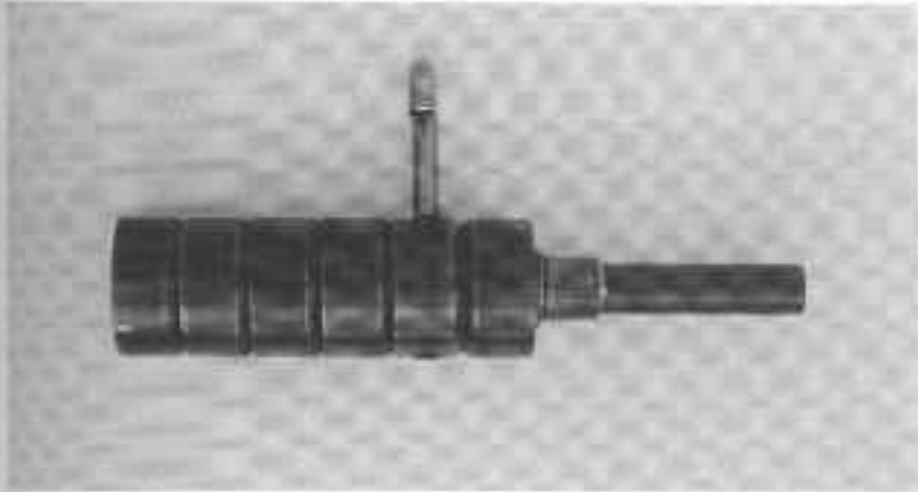
PHOTO 23: Breech block fully assembled with six collars and hook bolt in position.
