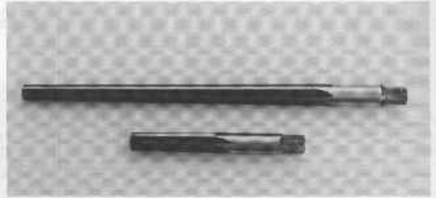
PHOTO 12: Taper pin reamer shown before and after cutting.
